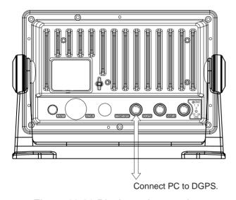
Figure 11-21 Display unit, rear view
